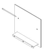
At hole center marks in template, drill holes using method A or B, depending on wall conditions as noted below:
