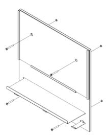
Slide lens and insert back in dry erase bracket and assemble magazine rack face, if existing, to bracket using cap and set screw assemblies. Not all models have slide-in lens or rack configurations. Remove finger prints from sign faces and edges using recommended cleaners. DO NOT use ammonia or alcohol based cleaners.
