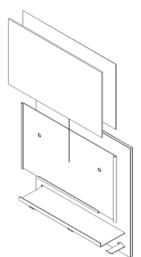
Tape template on wall at desired location, using a level to ensure template is level/plumb.
