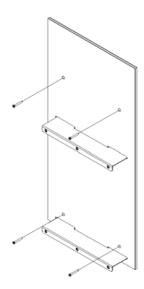
Attach each Magazine Rack front to bracket at (3) hole locations using cap and set screw assemblies. Use #50 hex key to tighten cap and set screw assembly snug against front panel.
