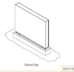
\*Important: When installing sign, it must be aligned and centered to foundation and surrounding design elements (ex: sidewalks, curbs, building fascia).
