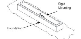
Install sign to foundation using flat washers, lock washers and socket head cap screws provided, aligning mounting plate hole locations on bottom of sign with anchors. Use level to ensure sign is level/plumb. Shims (not provided) may be required to level sign if foundation is not level. For a clean finish, ensure shims are not showing. Optionally, grout under flange.
