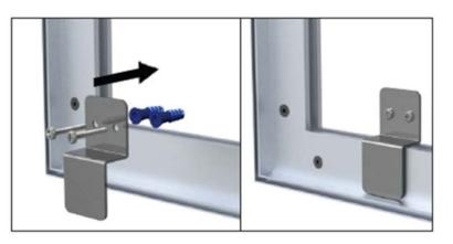
Wall Mount Brackets Distortion Brackets (if supplied) Assembly and Wall Mounting Screws Wall Anchors
