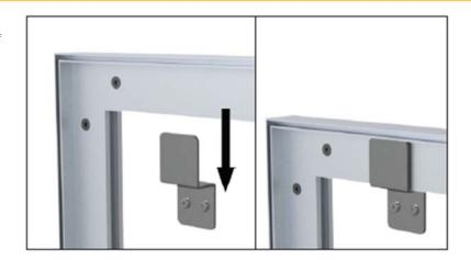
Position bottom row of wall mount brackets level on wall and mark mounting hole locations. Install wall anchors into masonry or drywall. Mount brackets onto wall using screws to complete secure mounting of frame assembly to wall.
