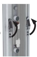
Connect corner pieces next by using catch and loops provided on extrusions. Repeat for other 3 corners.
