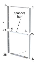
Connect straight pieces first. At each connection point, there should be 2 latches and 2 catches. Slide extrusion into its matching half. Then lift latch handle up and place loop over catch.
