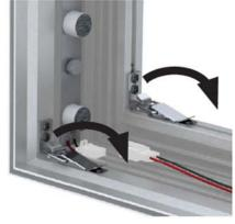
If spanner bar provided (typically for frames over 93"), place bar into frame channel and use thumb screw to expand end bracket inside spanner bar to secure it into frame channel.
