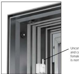
Unconnected and capped last female connector is normal
