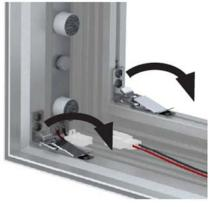
If spanner bar provided (typically for frames over 93"), place bar into frame channel and use thumb screw to expand end bracket inside spanner bar to secure it into frame channel.
